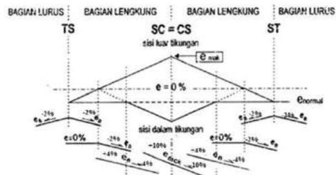
**Gambar 3.** Diagram Superelevasi Tikungan 1 (*Spiral-Spiral*)
