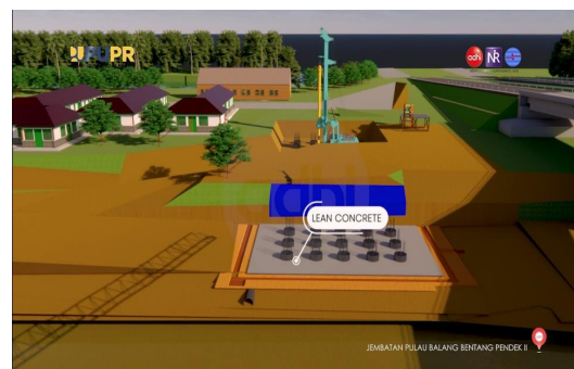
Gambar 3.7 Pekerjaan Lean Concrete Beton F_c'=10 MPa
