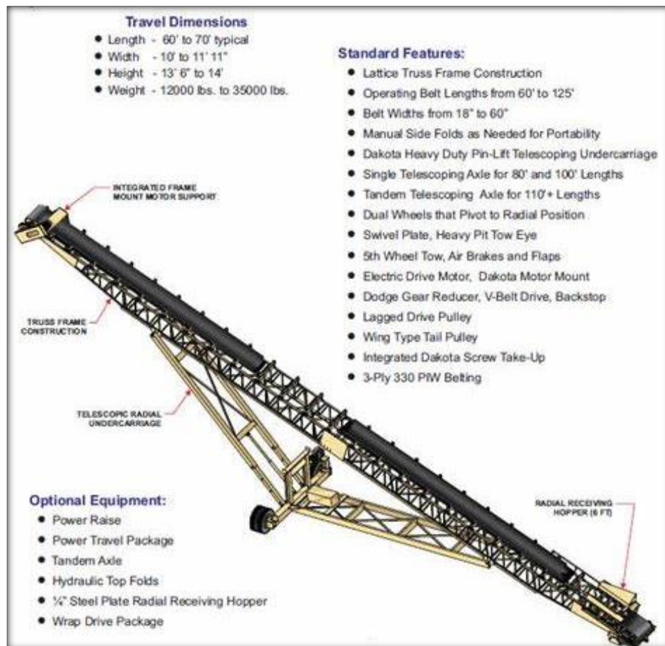
Gambar 2. 7 radial stacker conveyor
