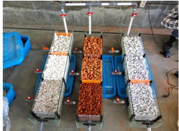
Gambar 3.1 Unit Horizontal Roughing Filter
