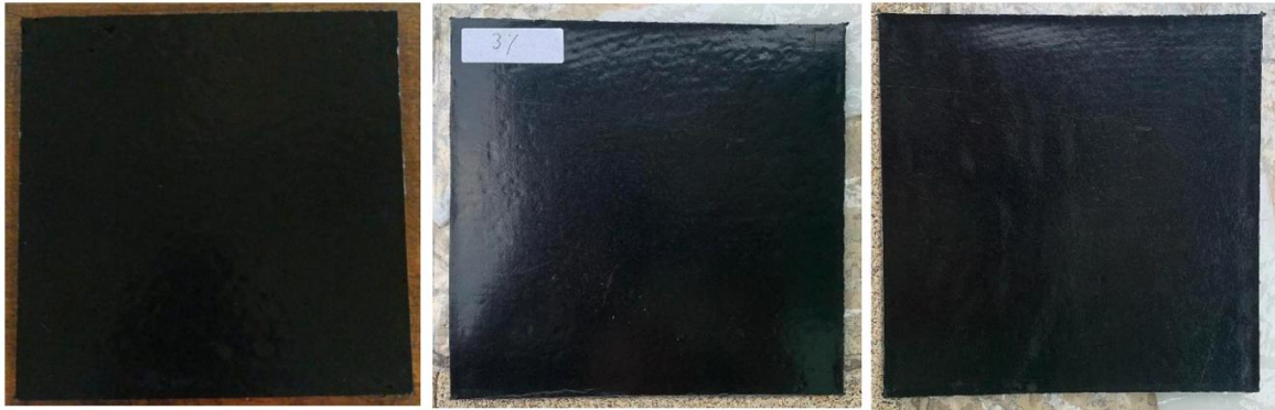
Figure 1. Recycled polypropylene (rPP) composites containing 0%, 3%, and 5% CTAB-modified bentonite after molding
