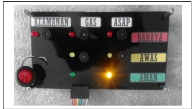
Gambar. 10. Panel Sistem Monitoring
